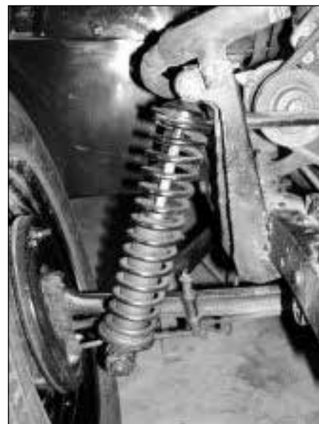
Photo 6: the Ashley's modified front suspension
