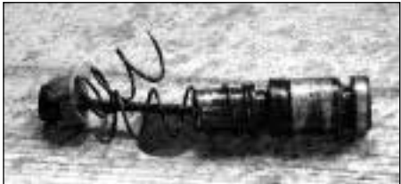
Photo 1: the broken master cylinder spring
