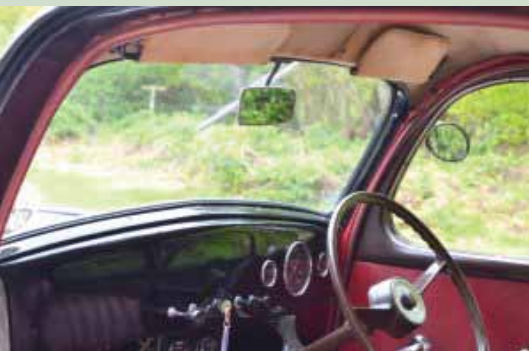
The Pop came minus any dash, just a sheet of painted steel fitted with dials.
