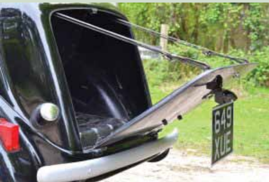
Straps secure the lid and the fold-down number plate allows travel loaded up with boot open.
