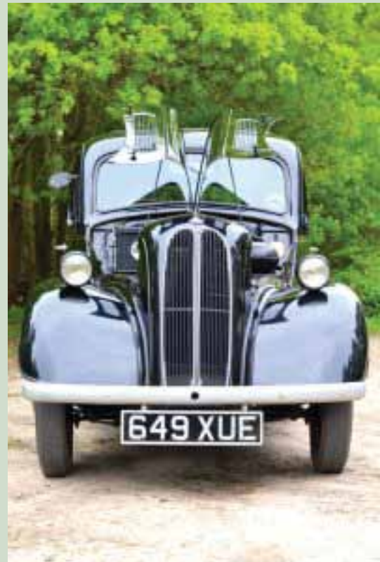
Double-sided bonnet opening and silver-painted bumpers, complete with space for starting handle.
