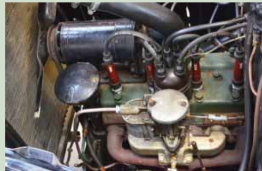
In-line four 1172cc sidevalve with single Zenith carb. Performance figures are irrelevant.
